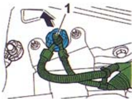
< Figure 1 > Loosening the ground straps.
