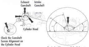
Check the Alignment of the Exhaust Camshaft Tone Ring. If Damaged or Out of Specs, Replace the Camshaft Assembly.
